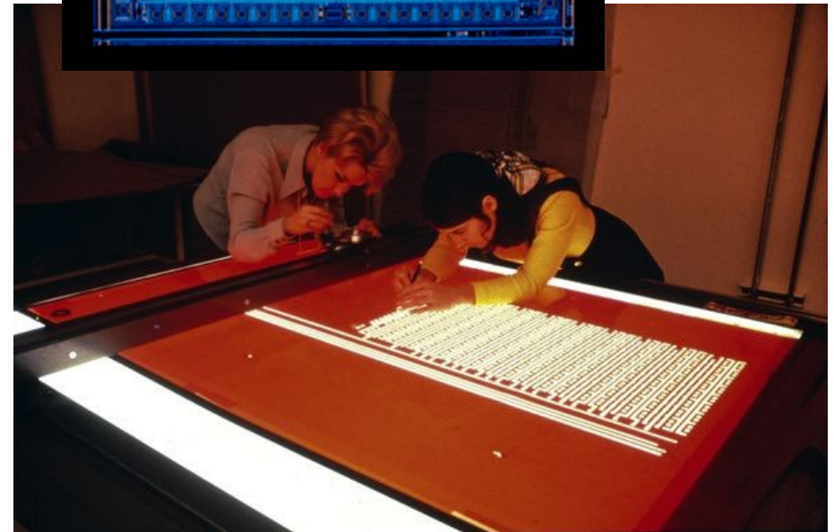
Operators hand-cut IC designs into Rubylith film, which is then optically reduced to a photolithography mask. (Intel, 1991)
