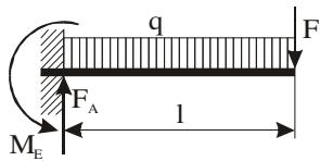
Print the following table of shear force and bending moment over x:
