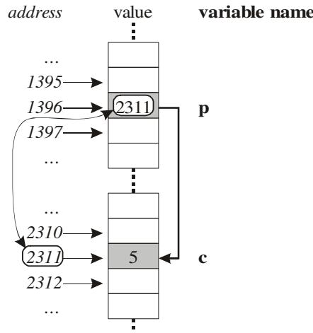
The unary operator `&` gives the address of an object (**address operator**), so the statement
