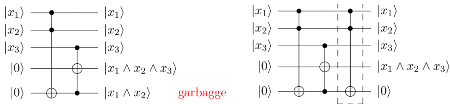
Figure 1: Example of garbage in an AND computation of x_1 \wedge x_2 \wedge x_3 and the uncomputation
