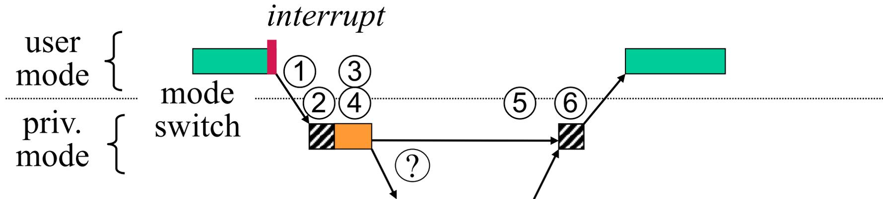
1. PC  $\rightarrow$  stack, ...; load PC from interrupt vector [HW]
