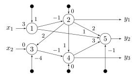
The numbers beneath the arrows denote the respective weights. Nodes 1 and 3 have the *identity* function as their activation function. Nodes 2 and 4 use the hard limiter with threshold 0 and node 5 uses a sigmoid function  $(1/(1+e^{-x}))$ . The arrows from the black dots give the respective bias weights. What is the output produced by the network when the input is  $(x_1, x_2) = (1, 1)$ ?
