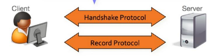
Provides confidentiality and authenticity of application layer data using keys from Handshake Protocol
