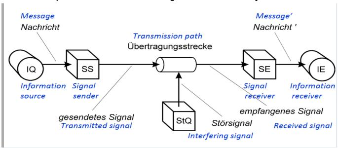
Difference between: message(identical sent and received) and transmission signal Deviations: impaired sender/receiver and path disturbance.
