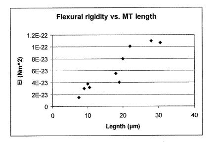
clearly EZ is not constant with length in these experimental data. Potential sources of error include: - reliable identification of initial buckling load - microtubles are not loaded directly in compression (bead twisting may occur)
