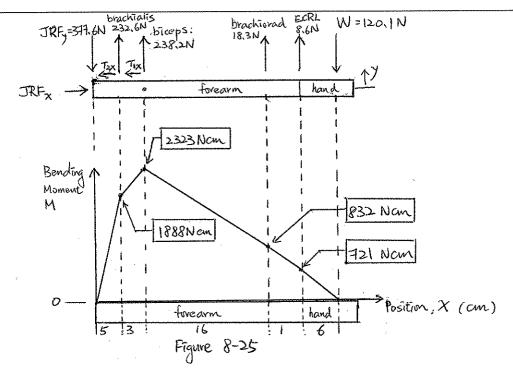
The axial stress due to the bending moment, M(x), and compressive internal force,  $F_x(x)$  is given by  $T(x,y) = \frac{M(x) \cdot y}{I_z} + \frac{F_x(x)}{A} \quad (eg'n \ 8.17)$
