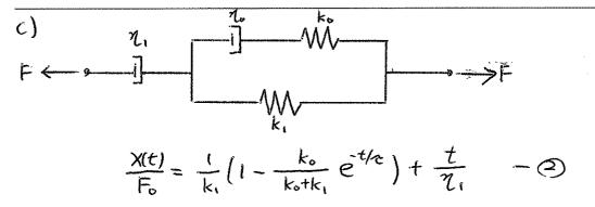
We are interested in the response at time  $t=0^+$ , where  $\chi = 0.95 \,\mu m$  (given) and  $F_5 = \frac{B}{Z} = \frac{200 \,nN \,\mu m}{50 \,\mu m} = 4 \,nN$
