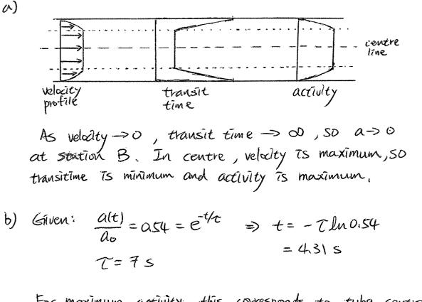
For maximum activity, this corresponds to tube centre line regim, T.e. U core. Also, blood travels 10 cm in 4.31 seconds, .'.  $U_{core} = \frac{10 \text{ cm}}{4.31 \text{ s}} = 2.32 \text{ cm/s}$
