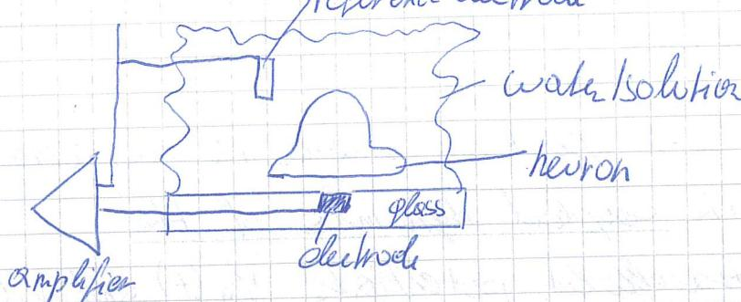
electrode in solution (electrochemistry)
