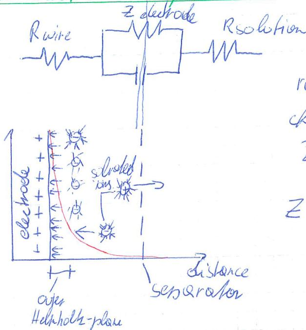
real electrodes are characterized by the impedance
