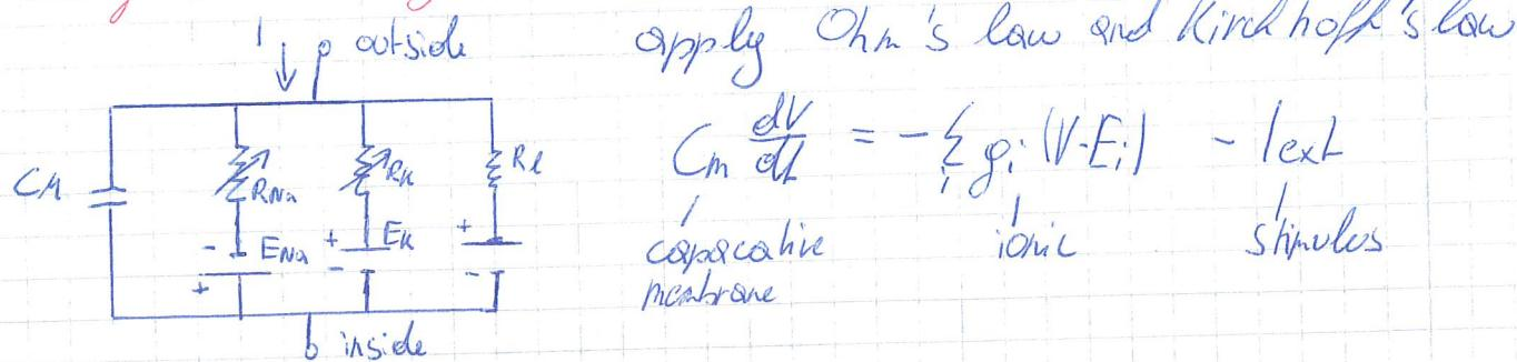
$$-C_m \frac{dV}{dt} = g_L (V - E_L) + g_K h^4 (V - E_K) + g_{Na} m^3 h (V - E_{Na}) + I_{ext}$$
