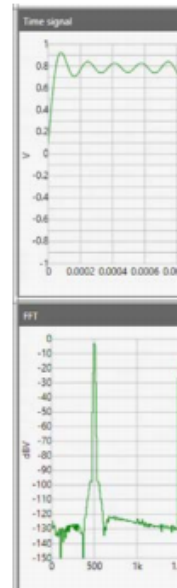
Fourier transform of bass guitar time signal of open string A note (55 Hz).
