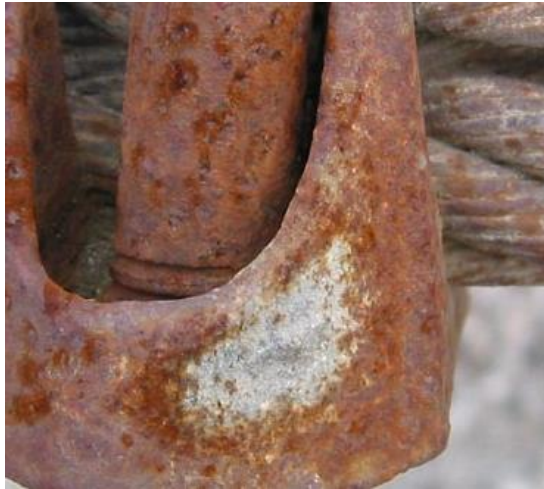
rust: ferrihydrite \text{Fe}_2\text{O}_3 \cdot n \text{H}_2\text{O}
