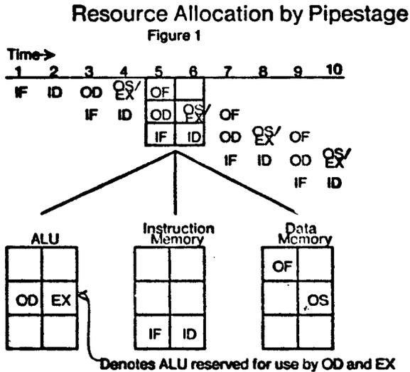
To achieve 100% utilization primitive operations in the microengine (e.g., load/store, ALU operations) must be completely packed into macroinstructions. This is not possible for three reasons:
