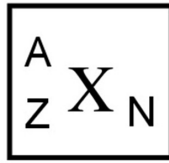
Figure 12: A... mass number / number of protons and neutrons Z... atomic number / number of protons N... number of neutrons (A-Z) X... Symbol of element.
