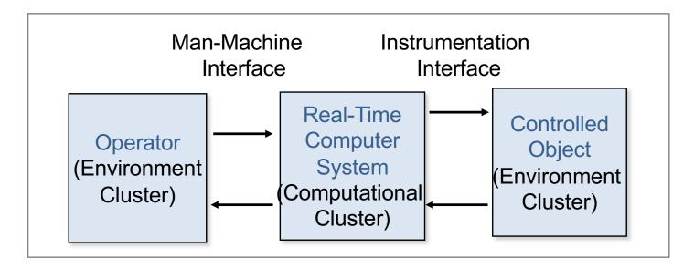
RTS: Controlled Object + Computer System + Operator
